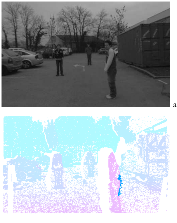
Figure 1: Left-side image from a stereo camera (a) and a corresponding disparity map (b)
