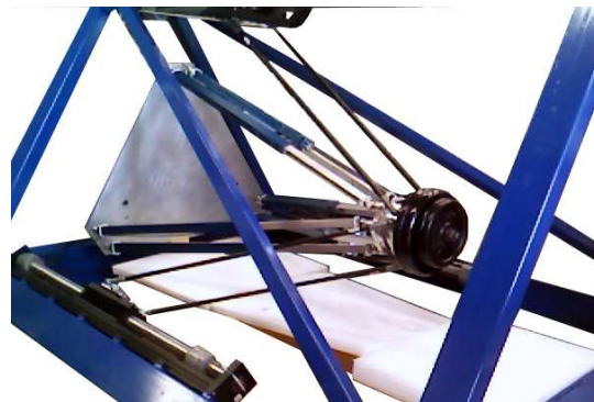
Figure 18: 140 N load applied on the MoM3 traveling plate
