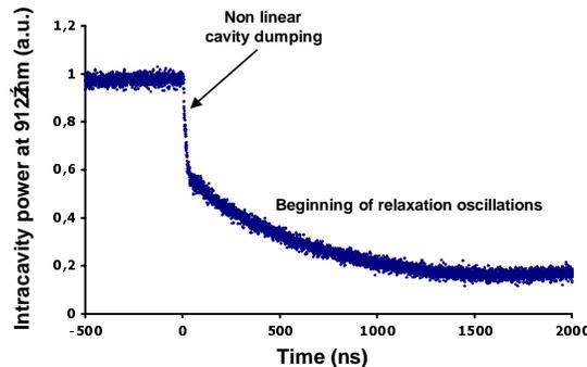
Fig. 3. Zoom on the intracavity power close to the nonlinear cavity dumping.
