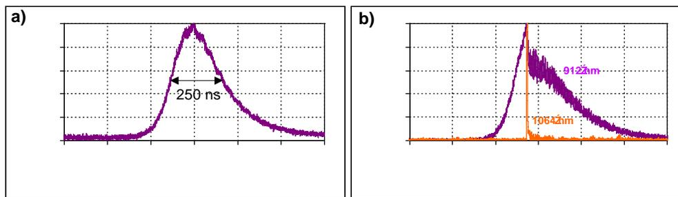
Fig. 5. (a) Pulse duration at 912 nm from the Nd:GdVO<sub>4</sub> Q-switched laser. (b) Temporal evolution of the intracavity power at 912 nm during the cavity dumping process.
