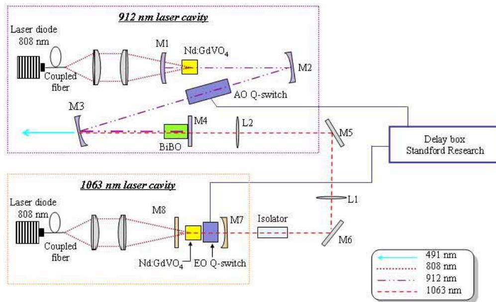
Fig. 1. Experimental setup. M1 radius of curvature is 50 mm, M2 radius of curvature is 200 mm, M3 radius of curvature is 200 mm, M4 is a plane mirror, M7 radius of curvature is 50 mm.
