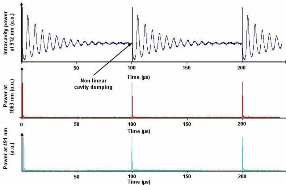
Fig. 2. Power recorded at 912 nm (intracavity, top), at 1063 nm (middle) and 491 nm (bottom) versus time.
