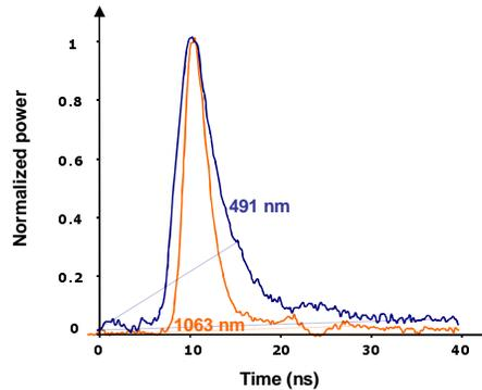
Fig. 4. Temporal pulse shape at 1063 nm and 491 nm obtained with the nonlinear cavity dumping process in case of a cw 912 nm laser. Secondary peaks are due to the pulse response of the photodiodes.
