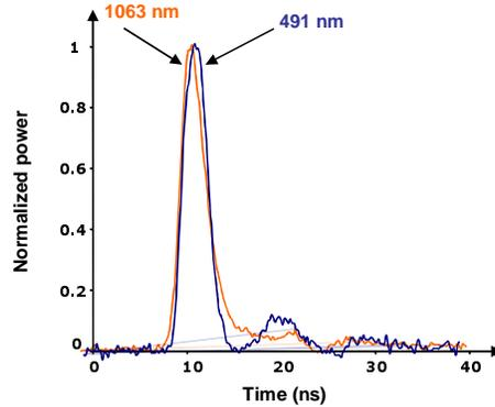
Fig. 6. Temporal pulse shape at 1063 nm and 491 nm from the nonlinear cavity dumping configuration with the Q-switched 912 nm laser. Secondary peaks are due to the pulse response of the photodiodes.
