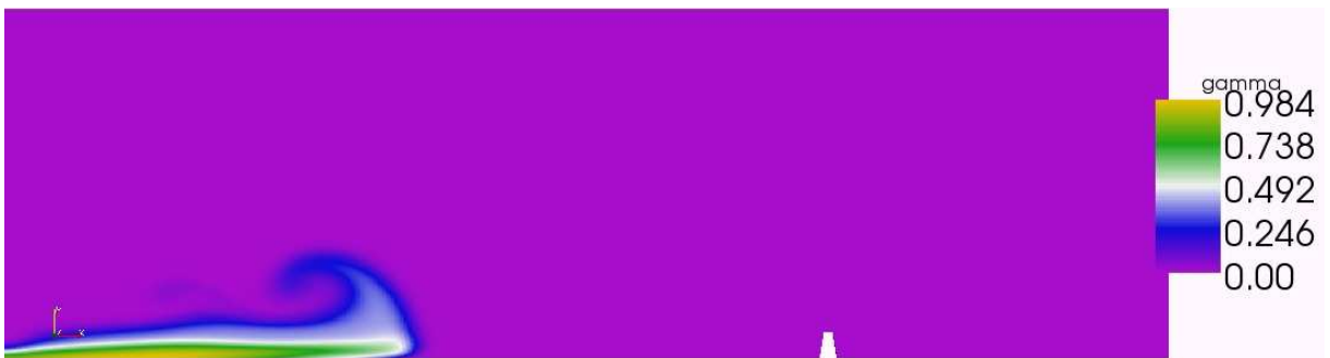
FIGURE 6. Avalanche at t = 25 s. The color scale ranges from 0 to the maximum value 0.984.
