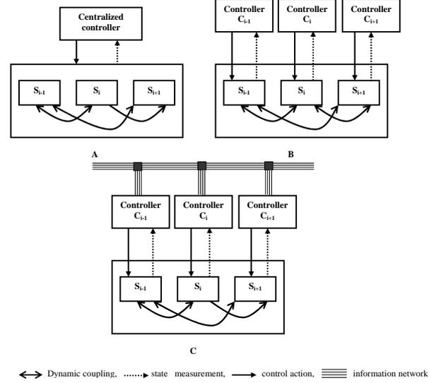
Fig. 1. A schematic representation of: A) Centralized control, B) Decentralized control C) Distributed control.
