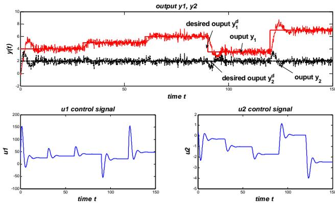
Fig. 3. Output responses with controllers implementing the proposed distributed MPC/KF coordination strategy.
