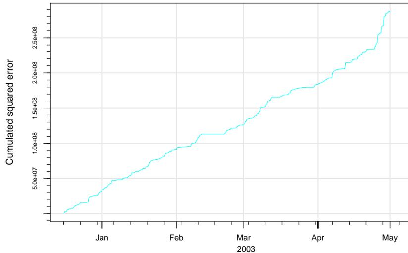
Figure 3: CUMULATED SQUARED PREDICTION ERRORS FOR THE TUNØ OFF-SHORE WIND FARM
