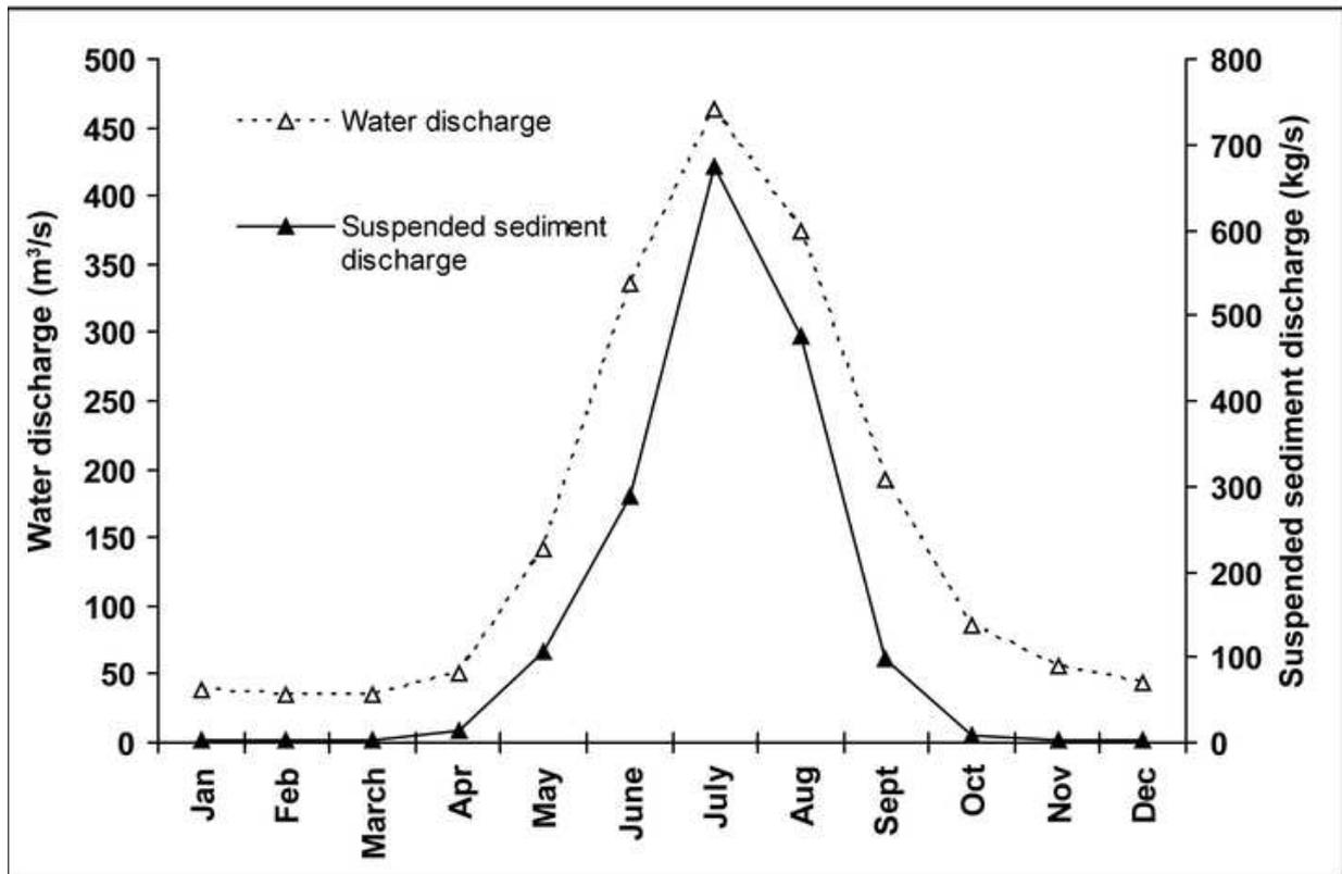
Fig. 2 Diagram of water discharge versus sediment discharge of Akdarya River (Uzdavsuvloixa, 2002)
