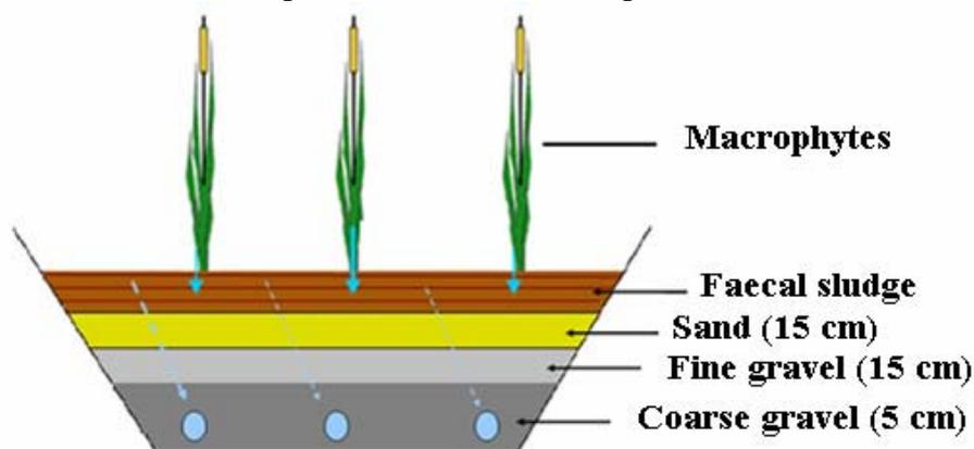
Figure 1: Diagram of a planted drying bed
