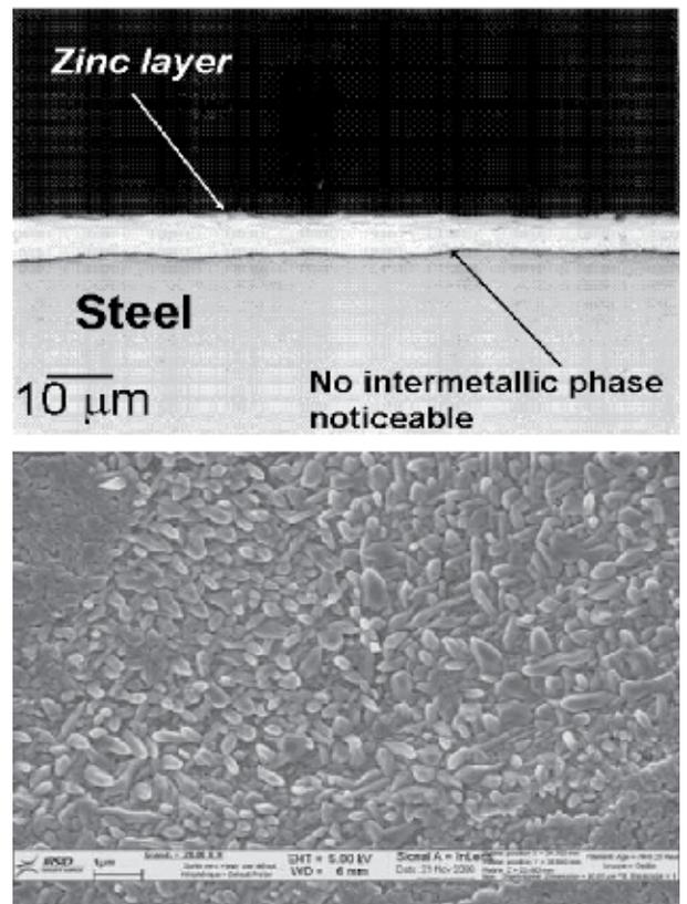
Fig. 2 - Optical cross section of GI coating (up); inhibiting layer as observed from the top, under SEM, after chemical stripping of the zinc layer (low).
