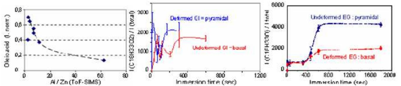
Fig. 10 – ToF-SIMS oleic acid peak as a function of surface Al on the left (immersion time: 600 s), and as a function of immersion time for un-deformed and deformed GI coating (centre) and EG coating (right). The solution was 1% oleic acid in hexadecane.
