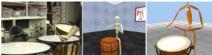
Figure 1.10: Synthesis of timpani gestures, based on motion capture data and a dynamical model of avatar
