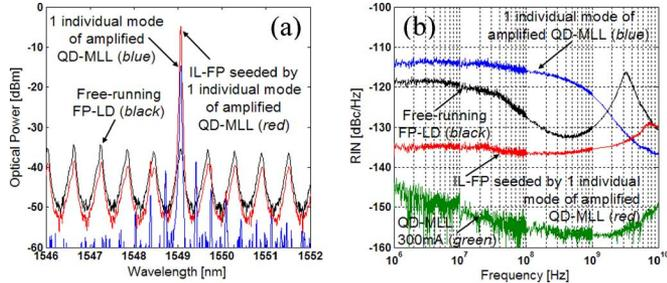
Fig. 2. (a) Injection-locking spectra and (b) RIN.
