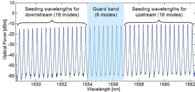
Fig. 1. Optical spectrum of QD-MLL at 300-mA bias.
