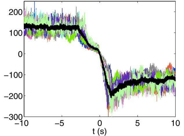
Fig. 4: Superimposition of 6 successive reversals from up to down polarity together with 6 successive reversals from down to up polarity with the transformation  $B \rightarrow -B$ . For each of them the origin of time has been shifted such that it corresponds to  $B = 0$ . The thick black line is the average of all reversals.
