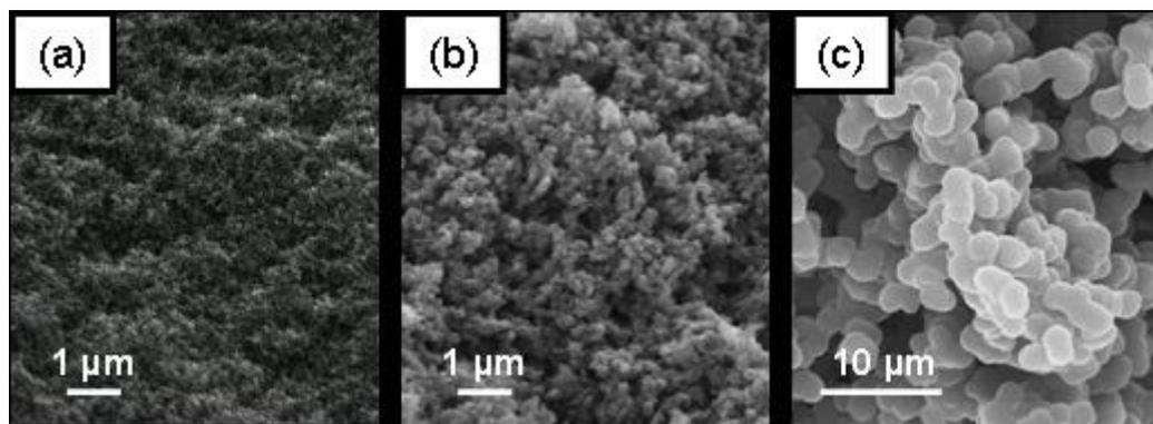
**Fig. 1** : Morphology of carbon xerogels prepared at various pH: (a) pH = 6.50, (b) pH = 6.00, (c) pH = 4.00. The size of the carbon nodules is completely determined by the composition of the RF solution, and does not depend on the drying technique. However, the drying method may alter the material shrinkage upon drying.
