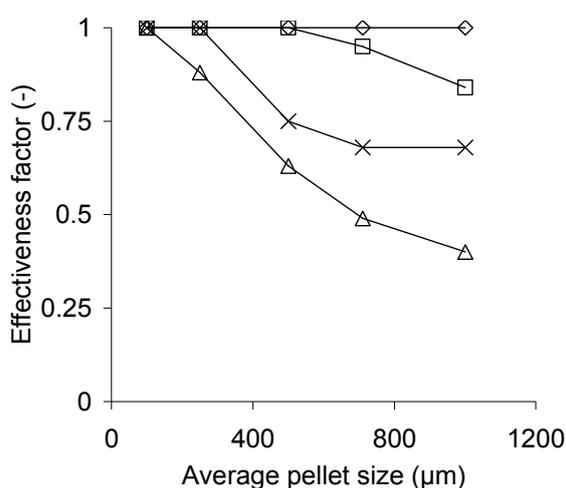
**Fig. 4** : Hydrodechlorination of  $\text{CH}_2\text{Cl}-\text{CH}_2\text{Cl}$  over Pd-Ag/carbon catalysts at 350°C in a fixed bed reactor: effectiveness factor as a function of the pellet size. Carbon xerogel supported catalysts: ( $\Delta$ ) small mesopores (8-10 nm), ( $\square$ ) large mesopores (25-30 nm), ( $\diamond$ ) macropores (60-70 nm). Catalyst supported on a microporous activated carbon ( $\times$ ). Data adapted from [14].
