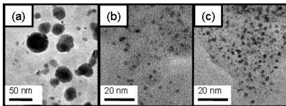
**Fig. 2** : Pt/carbon xerogel catalysts prepared on the same support (pore size range: 50 - 85 nm, pore volume = 2.1 cm<sup>3</sup>/g): (a) impregnation with  $\text{H}_2\text{PtCl}_6$  followed by direct reduction in liquid phase with  $\text{NaBH}_4$  (30 wt.% Pt [18]); (b) SEA method, one impregnation (7.5 wt.% Pt [23, 24]); (c) SEA method, three successive impregnations (22.7 wt.% Pt [24]).
