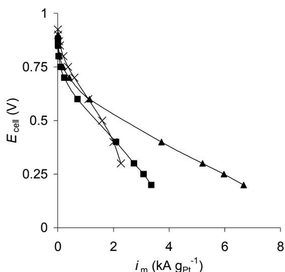
**Fig. 7** : Cell voltage vs. Pt mass activity. (■) carbon xerogel with small macropores (50-85 nm,  $2.1 \text{ cm}^3 \text{ g}^{-1}$ ), impregnation + liquid phase reduction [18]; (▲) carbon xerogel with small macropores (50-85 nm,  $2.1 \text{ cm}^3 \text{ g}^{-1}$ ), SEA method (double impregnation, reduction under  $\text{H}_2$  flow at  $450^\circ\text{C}$  [42]), (×) commercial cathode (Pt/carbon black, Paxitech).
