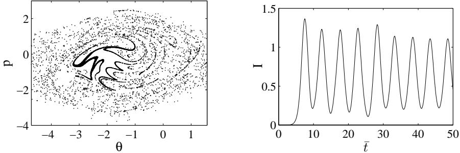
**Figure 1.** Left: Electron phase-space in the QSS regime (at  $\bar{t} = 50$ ). Right: Normalized laser intensity versus normalized time  $\bar{t}$ . Simulations performed with  $N = 8000$  particles, starting with a waterbag with  $b_0 = 0$ ,  $\Delta p = 0.05$ , and a negligible intensity  $I_0 = 10^{-6}$ .
