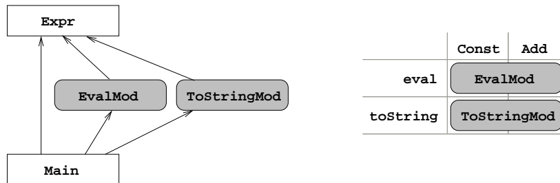
Figure 2: Constructor decomposition (architecture of the program P_{data} )
