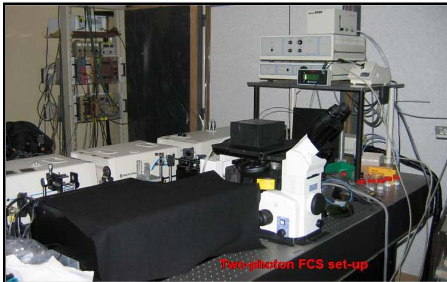
**Figure 16 : Instrumentation of two-photon FCS.**
