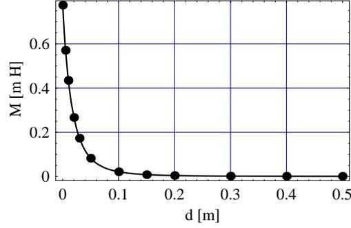
**Figure 4.** Representation of the mutual inductance between two thick coils versus the axial distance  $d$ ;  $r_1 = r_3 = 0.025$  m,  $r_2 = r_4 = 0.03$  m,  $z_2 - z_1 = z_4 - z_3 = 0.025$  m,  $N_1 = N_2 = 200$ .
