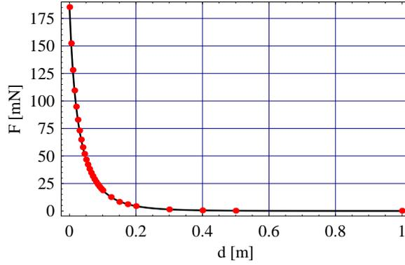
**Figure 2.** Representation of the axial force exerted between two thick coils versus the axial distance  $d = z_3 - z_2$ . We take the following dimensions:  $r_1 = r_3 = 0.0875$  m,  $r_2 = r_4 = 0.1125$  m,  $z_2 - z_1 = z_4 - z_3 = 0.025$  m,  $j_1 = j_2 = 320\,000$  A/m<sup>2</sup>. Line = our analytical method, Points = Filament method
