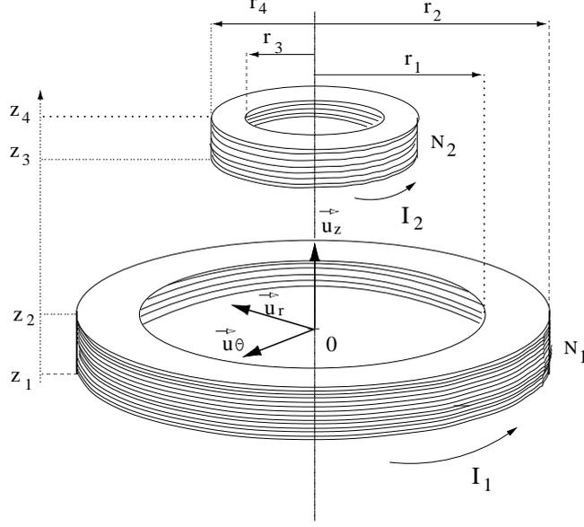
**Figure 1.** Geometry considered: two thick coils carrying uniform current volume densities. For the lower thick coil, the inner radius is  $\mathbf{r}_1$ , the outer one is  $\mathbf{r}_2$ , the lower height is  $\mathbf{z}_1$ , the upper one is  $\mathbf{z}_2$ ; for the upper thick coil, the inner radius is  $\mathbf{r}_3$ , the outer one is  $\mathbf{r}_4$ , the lower height is  $\mathbf{z}_3$ , the upper one is  $\mathbf{z}_4$ .
