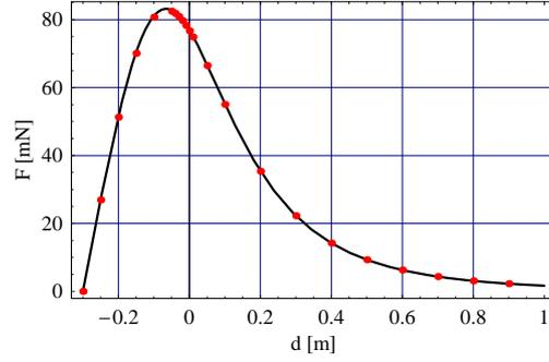
**Figure 3.** Representation of the axial force exerted between two toroidal conductors versus the axial distance  $d$ . We take the following dimensions:  $r_1 = r_3 = 0.0875$  m,  $r_2 = r_4 = 0.1125$  m,  $z_2 - z_1 = z_4 - z_3 = 0.025$  m,  $j_1 = j_2 = 320\,000$  A/m<sup>2</sup>. Line = our analytical method, Points = filament method.
