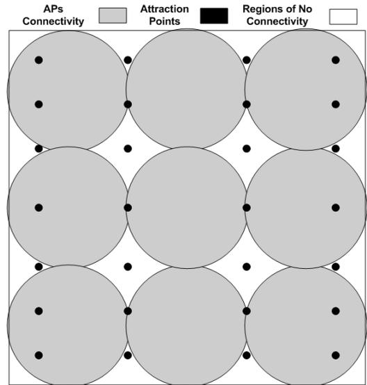
Figure 6 Uniform Deployment of 9 APs (28 Attraction Points)
