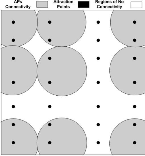
**Figure 8 Non-uniform Deployment of 9 APs (28 Attraction Points)**
