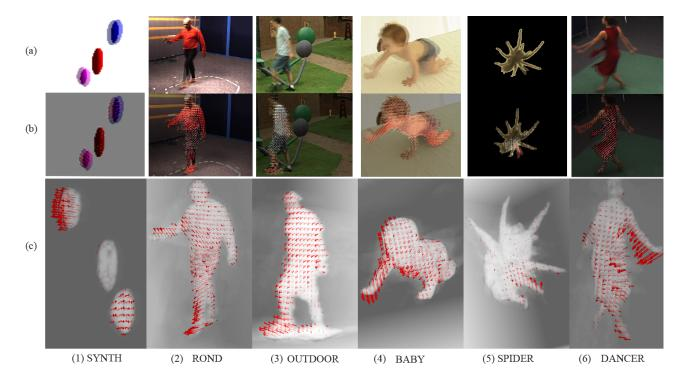
Figure 3. 3D occupancy flow result (**Best viewed in color**). Six datasets are illustrated column-wise. (a) The overlaid consecutive frames to indicate the motion; (b) the motion field on top of the respective image in (a); (c) the motion field and the occupancy probability grid from a novel view. Fig. 1 is part of the ROND dataset. Please check the supplementary video for the complete sequence results.
