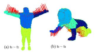
Figure 7. Rigid motion segmentation results (**best viewed in color**). Only voxels above probability 0.98 are used for this computation. (a) ROND result using motion from  $t_0$  -  $t_2$ ; (b) BABY result using motion from  $t_0$  -  $t_6$ . Each rigid part is shown with a specific color. The rigid motion (translation and rotation) of each part is shown in red vectors, which explains the real motion at the time instant properly.
