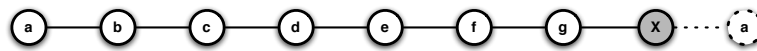
Figure 10: Link Spoofing: The malicious router X advertises a spoofed link to router a in its TC messages, thus all routers will record the links X-a and b-a .
