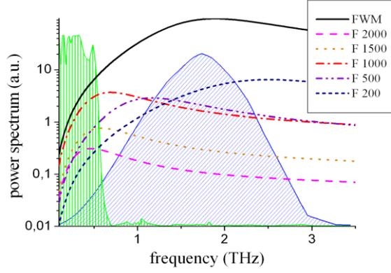
FIG 4. THz power spectrum extracted from the best fit to formula (1) for different focusing lenses  $F$ . The continuous line represents the fit for the Four Wave Mixing emission of a  $200 \mu\text{J}$  two-colour pulse. Also shown in dashed area are the transmission windows of the filters B and D (in arbitrary units).
