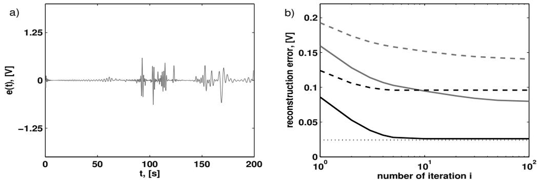
Figure 4: (a) The difference between original and recovered signal from its 349 level-crossing samples after 10 iterations and (b) reconstruction error (solid lines - reconstruction from level-crossings using  $h_2(t, t_n)$ , dashed lines - reconstruction from level-crossings using  $h_1(t, t_n)$ , dotted line - reconstruction from samples obtained by  $\Phi(t_n) = n\pi$ ).
