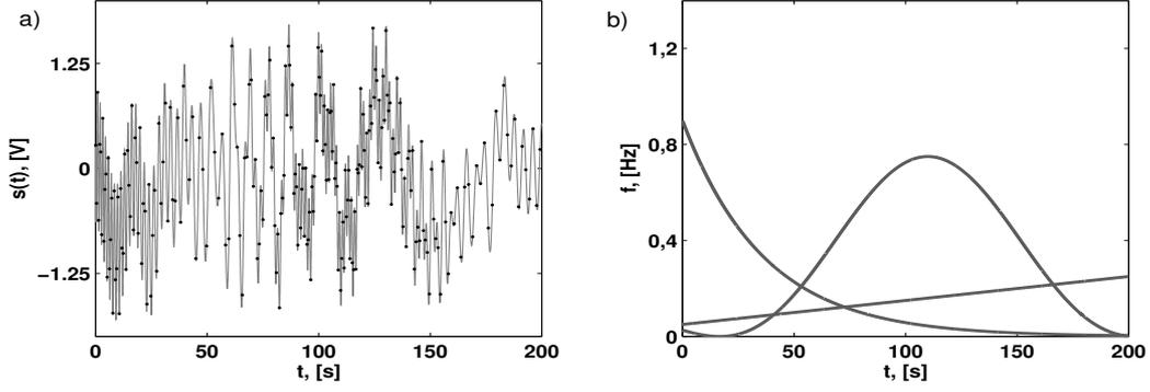
Figure 2: (a) Test signal sampled by  $\Phi(t_n) = n\pi$  and (b) frequency traces of its components.
