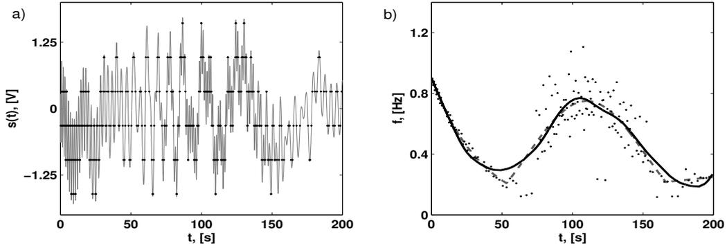
Figure 3: (a) Test signal sampled by level-crossings and (b) estimated instantaneous maximum frequency  $\hat{f}_{max}(t)$  as solid line, true instantaneous maximum frequency as dashed line and  $f(t_j)$  as black points.
