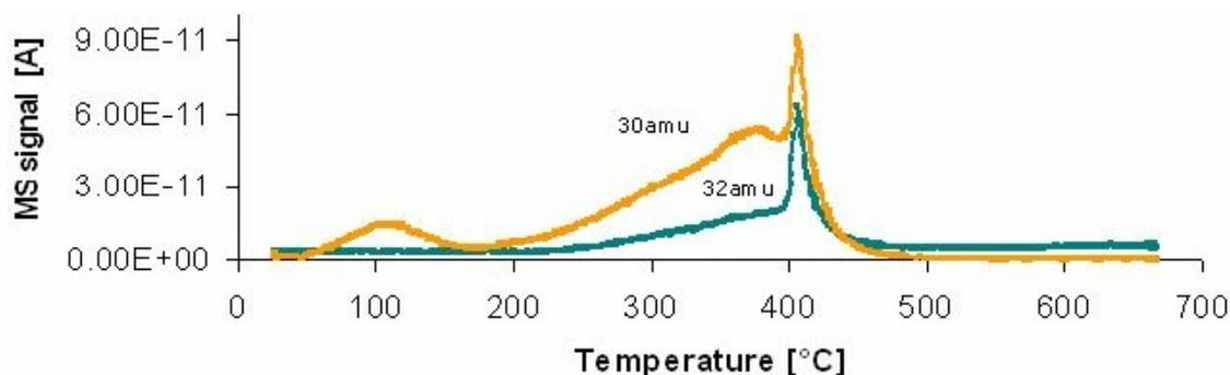
Figure 5. TPD profile of 1.7%Pt dispersed in alumina for NO<sub>x</sub> ions (at 30 amu) and O<sub>2</sub><sup>+</sup> (at 32 amu)
