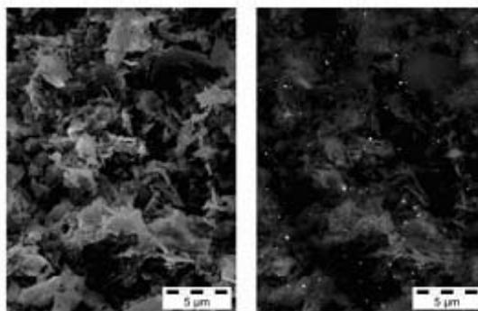
*Figure 6. SEM images of the catalytic filter surface (1.7%Pt dispersed in alumina)*
