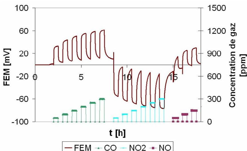
*Figure 3. Sensing characteristics of a Au/YSZ/Pt sensor without a catalytic filter layer at 450°C in presence of 12% O<sub>2</sub>*
