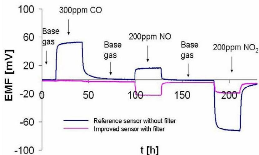
Figure 4. Sensor response to CO, NO and NO<sub>2</sub> at 520°C (Base gas: 12vol.% O<sub>2</sub>, 2vol.% H<sub>2</sub>O, N<sub>2</sub> balance)
