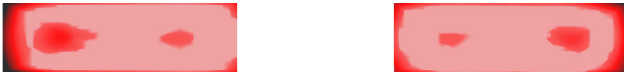
Fig. 2. Current displacement in the conductor cross section of the two turn side of the test inductor. Plot obtained by HFSS-simulation of the test-inductor, current density in logarithmic scale increasing to darker colors (see figure 3). The slightly higher current in the very inside of the metal is due to small simulation inaccuracies.
