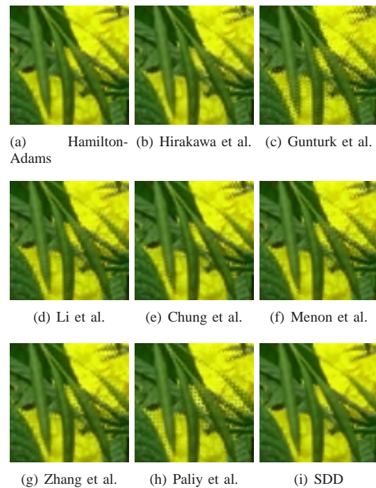
Figure 10. Zipper effect on IMAX images. Most methods present a strong zipper effect on color edges that makes the demosaicked image not a reasonable solution to the demosaicing problem. Only the SDD algorithm and Hamilton-Adams are able to give a reasonable solution.
