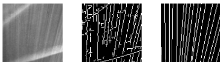
Figure 12: Example of results obtained when a canvas tarpaulin is used for the background. Left side: grey level image (detail); middle: binary image (detail); right side: identified trajectories.
