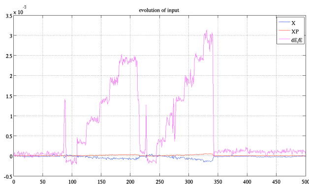
Figure 4: Evolution of x, x' and dE/E reconstructed at the injection point.
