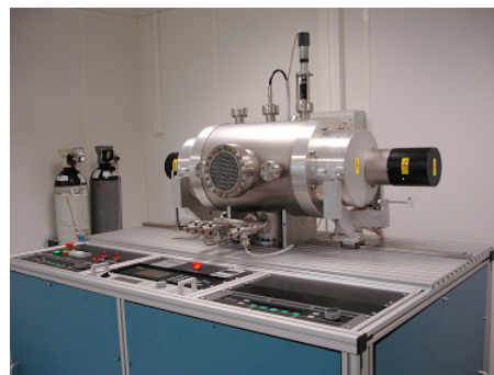
Figure 1: Sputtering system Overview.
