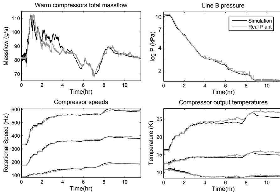
Figure 10: Comparison between experimental and simulated main variables during the pumping from 10 kPa to 1.6 kPa of a LHC sector
