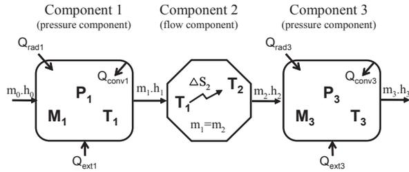
Figure 4: Connections between flow and pressure components
