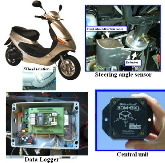
Figure 12. Motorcycle equipment using for validation.
