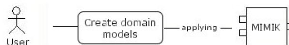
Fig. 5. Context diagrams are almost exactly the same as use cases in UML, with the addition of the concept of knowledge packet.
