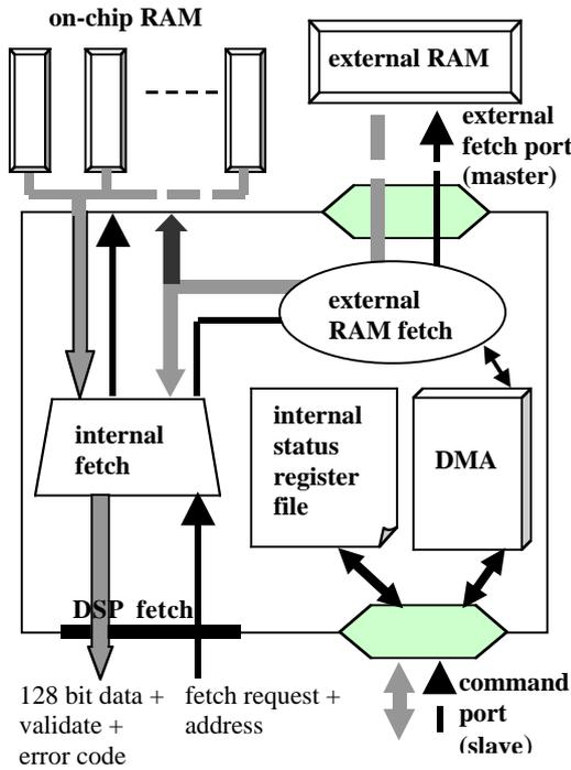
Figure 1 - Architecture of the cache controller
