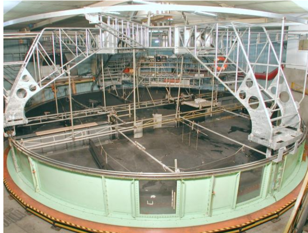
Figure 5: The Coriolis rotating platform at Grenoble equipped with the translation carriage along the diameter
