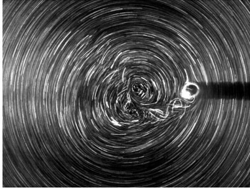
FIGURE 6. Long-time exposure for a large bubble ( Re > 100 ). Ro < 6 . Strong coupling between the bubble, the flow and two co-rotating vortex occurs with a 2\omega frequency. This frequency can be seen as the signature of that coupling, so, no forces are measured when it appears in the spectrum of the bubble locations around equilibrium.
