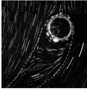
FIGURE 11. Visualization of a bubble and its wake. The visually estimated edges of the wake have been materialized with a dashed line. d_b \approx 1 mm, Re \approx 120 , Ro \approx 8 , \Omega_b/\omega \approx 1.4 . The near wake appears to be quite large. This must have an impact on the drag, increasing it.
