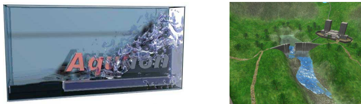
Figure 4: Dam break flow over an obstacle (left)-Dam break flow on a realistic topography (right)
