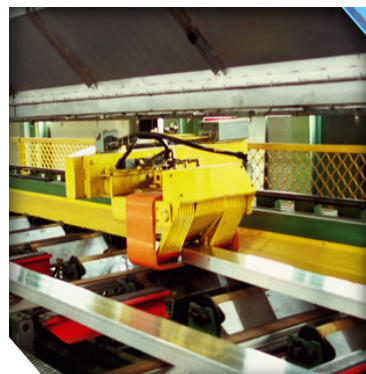
Figure 3: Run out table and puller
