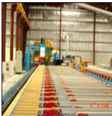
Figure 3: Run out table and puller
