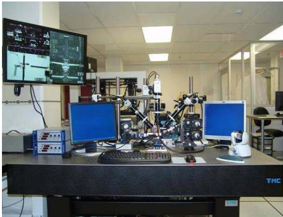
Figure 1: \mu^3 microassembly system at ARRI's Texas microfactory
