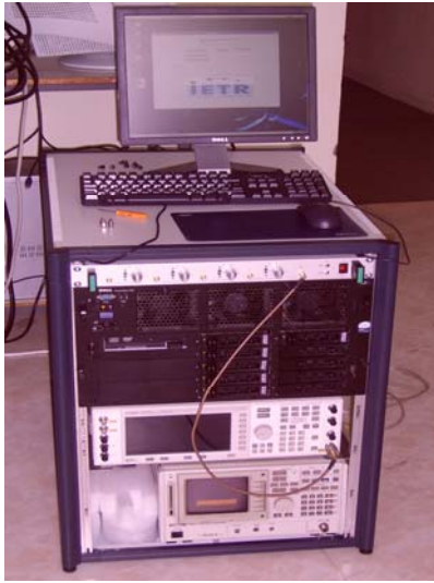
Fig. 3 Receiving and acquisition system
