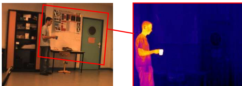
Figure 3: Spatial registration of the visible video (left) on the IR video (right). The red rectangle is the field of view common to both sequences.
