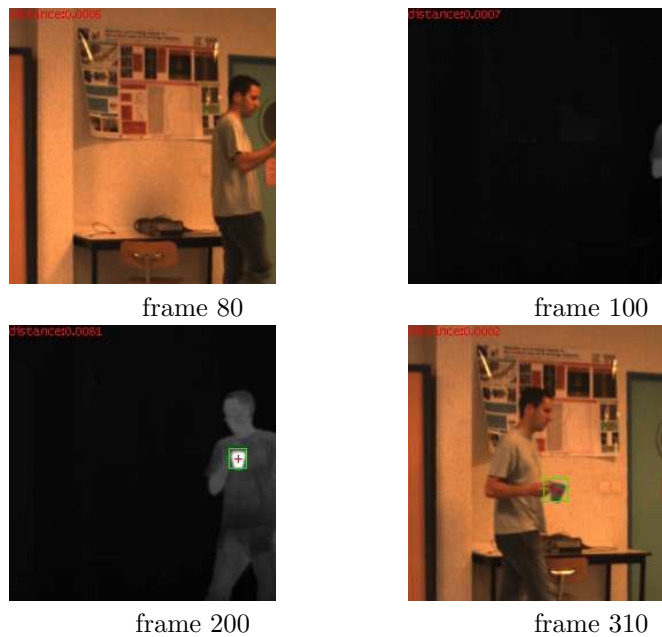
Figure 6: The “coffee cup” sequence: cooperative tracking using visible and IR video. Frames in grayscale (100 and 200) originate from the IR video while frames 80 and 310 originate from the visible camera. IR video assumes tracking after switching off the lights and continues until lights are switched on. Then the visible video assumes tracking again.
