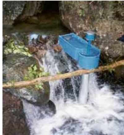
Figure I.4 : Petite turbine hydraulique de 200 W [I.7]
