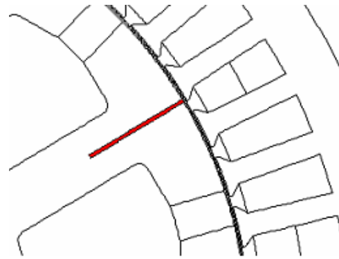
Fig. 17. Slit in the pole
