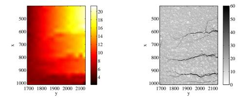
Figure 6. Vertical displacement expressed in pixels (left) and gray level residual map (right) revealing a complex multiple crack pattern (1 pixel =  $370 \ \mu$ m).
