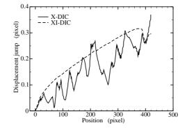
Figure 11. Normal displacement discontinuity across the crack face as determined with the eXtended Q4-Digital Image Correlation (solid line: X-DIC) and using the elastic regularization (dashed line: XI-DIC). 1 pixel =  $1.85 \ \mu m$ .
