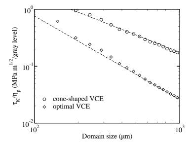
**Figure 15.** Uncertainty of the determination of the SIF for the optimal VCE (symbol  $\diamond$ ), when compared to a reference case (*i.e.*, the cone shaped VCE symbol  $\circ$ ), as a function of the domain size for the SiC case (mode I). The dotted lines are power-laws of slope -1, and -3/2.
