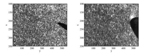
Figure 3. Reference (left) and deformed (right) pictures of a crack in a rubber specimen (courtesy of S. Mzabi). The pixel size is 9.38  $\mu$ m.
