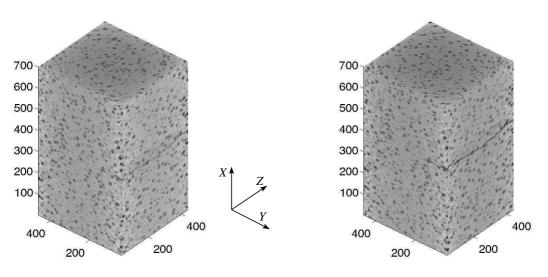
Figure 18. Reference (load 5 N) and deformed (load 100 N) 3D images of a cracked sample. The load is applied along the longitudinal direction (normal to the crack). The voxel size is  $3.5 \ \mu m$ .
