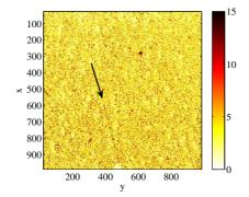
Figure 7. Residual field for the SiC sample shown in Figure 1. It is expressed in difference of gray levels between the reference and corrected deformed images, and should be compared to the full dynamic range of the image (210 gray levels).
