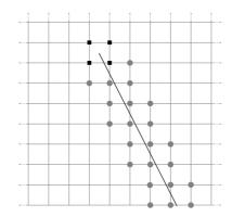
Figure 9. Schematic plot of the regular Q4 mesh, the nodes (shown as gray disks) supporting a discontinuous enrichment, and the nodes (shown as black squares) supporting a singular (crack-like) field.
