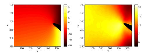
Figure 4. Vertical (left) and horizontal (right) components of the displacement for the crack in rubber. The displacement field has been decomposed over Q4 elements whose size is  $\ell = 32$  pixels. The color scales for the displacements are expressed in pixels (1 pixel = 9.38  $\mu$ m).
