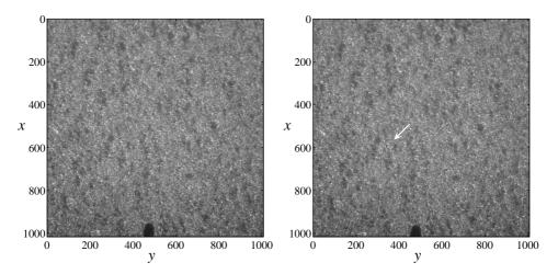
Figure 1. An example of a SiC sample prior to (left) and after (right) crack propagation from the notch along the bottom side. The image texture is that of the natural surface roughness. The pixel size is 1.85  $\mu$ m. The white arrow indicates the position of the crack tip (which cannot be seen on this picture). The crack extends down to the notch that is located on the lower side.
