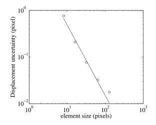
Figure 8. Standard uncertainty as a function of the element size  $\ell$  for a finite element decomposition of the displacement field when  $\Delta = 0.5$  pixel. A power-law decrease as  $A^{1+\alpha}\ell^{-\alpha}$  is typically observed, with  $A \approx 3$  pixels and  $\alpha \approx 1.5$  for the reference picture shown in Figure 1. An element size  $\ell = 32$  pixel (as used in the previous examples) leads to an uncertainty of the order of  $8 \times 10^{-2}$  pixel.
