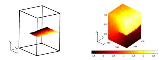
Figure 20. Geometry of the crack surface (left). Displacement component (expressed in voxels) along the loading direction obtained from Digital Image Correlation using an enriched kinematics (right). The volume shown here lies strictly inside the sample to avoid edge effects. The voxel size is  $3.5 \ \mu m$ .
