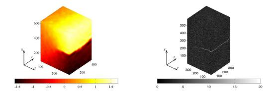
Figure 19. Displacement component (expressed in voxels) along the loading direction obtained from Digital Image Correlation using C8 elements whose size is  $\ell = 32$  voxels (left). Corresponding residual field (right). Its level should be compared to the dynamic range of the pictures (*i.e.*, 256 gray levels). The voxel size is 3.5  $\mu$ m.
