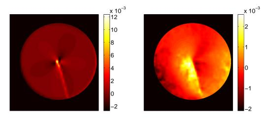
Figure 16. Horizontal component of the extractor field (normalized by  $2\mu\sqrt{p\pi}$  where p is the pixel size here equal to 1.85  $\mu$ m) for the interaction integral with a conical VCE(left) and with the optimal VCE (right).
