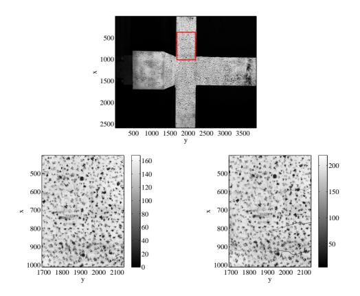
Figure 5. Large scale view of part of a reinforced-concrete frame (top), zoom on an analyzed region in its reference (bottom left) and deformed (bottom right) state. The pixel size is 370  $\mu$ m. Note that large cracks can be guessed in the deformed image in spite of the surface marking.
