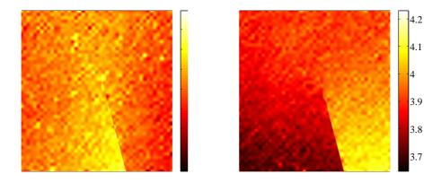
Figure 10. Vertical (left) and horizontal (right) components of the displacement field for the SiC sample of Figure 1 as resolved with the eXtended Q4-Digital Image Correlation. Q4 elements are used with a size  $\ell = 32$  pixels. The color scales for the displacements are expressed in pixels (1 pixel = 1.85  $\mu$ m).
