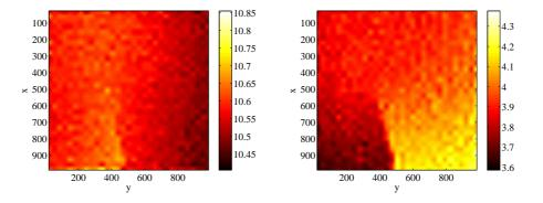
Figure 2. Displacement field for the SiC sample shown in Figure 1. The vertical (resp. horizontal) component of the displacement field is shown on the left (resp. right). The displacement field has been decomposed over square-shaped bilinear shape functions (Q4 in the language of finite elements) whose size is  $\ell = 32$  pixels. The displacements are expressed in pixels (1 pixel = 1.85  $\mu$ m).
