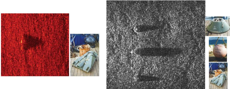
Fig. 2. On the left, SAS image and picture of the associated modern mine. On the right, SAS image and picture of the associated modern mines
