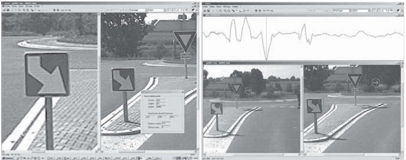
Figure 5 Graphic interface of the STEREO demonstrator software. Measurement of the dimensions of a J6 beacon (left); point-specific matching and diagram of (dis)similarity (right).
