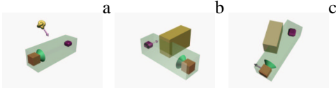
Figure 1: Occlusion issues (a) occlusion due to a moving object (b) occlusion due to the target motion (c) occlusion due to the camera motion
