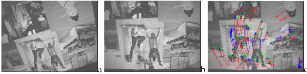
Figure 5. Visual servoing based on the tracking of points of interest: (a) initial image, (b) desired image, (c) robust visual servoing.
