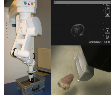
Fig. 7. Experimental setup: (left) ultrasound probe mounted on a 6 DOF medical robot - (right) Observed US image and the rabbit heart suspended in a water-filled box
