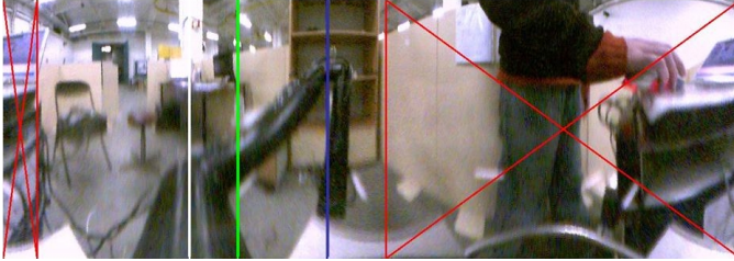
Fig. 4. Panoramic view provided to the user before the arm positioning. Red crosses: positions that can not reach the first joint. White line: first axis position. Blue line: initial FOV of the camera (left picture of Fig 3). Green line: desired camera direction, given by the user with one click. After the arm positioning, the embedded camera gives the right picture of Fig 3.
