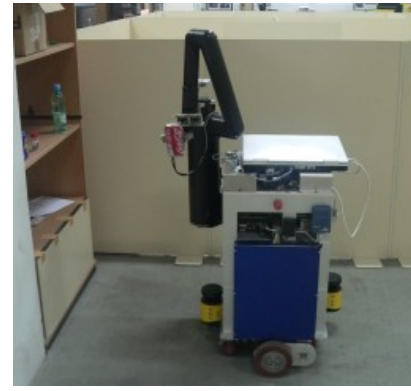
Fig. 1. SAM: a Manus arm mounted onto the MPM470 mobile platform.
