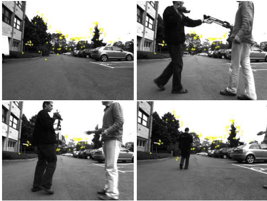
Fig. 9. Robust feature tracking resumption after occlusion during navigation in experiment 2.
