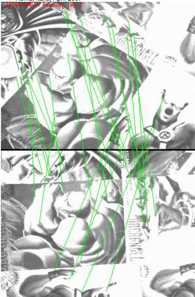
Fig. 5. Initial (top) and reference (bottom) image for the marvel experiment. Green lines link two matched point.
